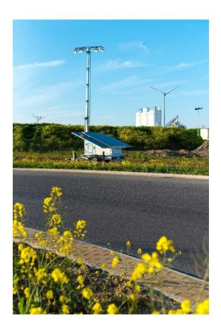
All ProLight solar units used on the A14 have been fitted with an upgrade that enables the works team to power 1800w hand tools with the solar energy generated and stored in the light's battery system. The enhancement has increased the team's ability to reduce carbon impact, as well as removing the noise and fumes of diesel generators.
